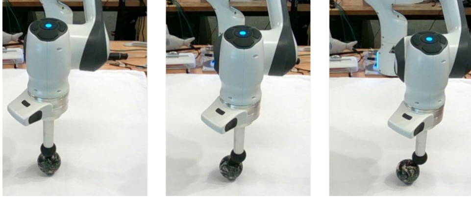
Figure 4.15: An example of a left to right roll using C3 as a high-level planner. Despite the provided heuristic, C3 positions the end-effector directly above the ball at the start of the motion (left image) and rolls from the front.
